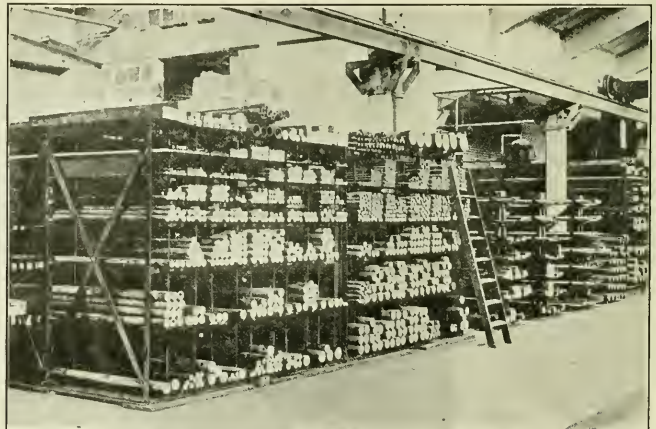
MATERIAL RACK WITH IDENTIFICATION COLORS PAINTED ON THE ENDS OF THE STEEL BARS.
